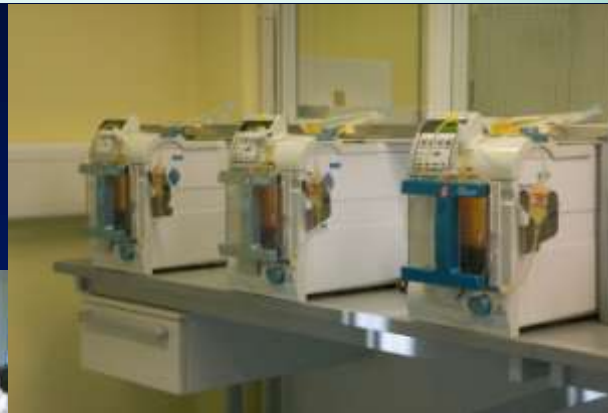
Separation of different blood layers for BC production
